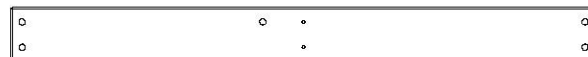
H8 | LISSE DE PLANCHER - W4L13295 (1) | 1 po x 3 3/8 po x 36 5/8 po (24 x 86 x 930)
